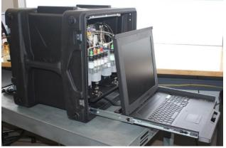
The 19" rack is equipped with a rack-mounted highintensity LCD screen to allow for outdoor use. A keyboard and pointing device is integrated into the screen's 1U shelf. A KVM (keyboard, video, and mouse) switch allows switching of the display between the NUC computers that drive the two FloPro-Analyzers. All devices in the rack are powered from a single 100-250VAC power strip.
