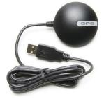
The Globalsat USB GPS receiver streams data in standard WGS-84 format which is easily converted to longitude and latitude and can be plotted on a Google Earth map (requires internet connection to acquire initial map space). If an Internet connection is not available, the data are plotted on an x-y grid scaled to the far extents of the location space of the chosen data set.
