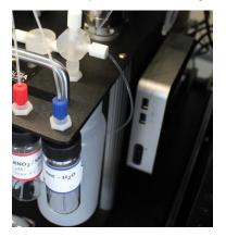
The software is installed on an Intel NUC computer which is mounted on the side of the FloPro. This compact computer is equipped with a 4<sup>th</sup> Gen Intel i5 processor and Windows 7 operating system. It's built in Wi-Fi means that the computer is accessible wherever Internet connectivity is available.
